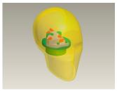
The Six Accelerometer Package (SAP) measures the linear and rotational accelerations of a mannequin headform in all six degrees of freedom for kinematics analysis or for use with head injury assessment functions.
