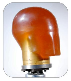
Elastomeric headform for ballistic limit assessment
