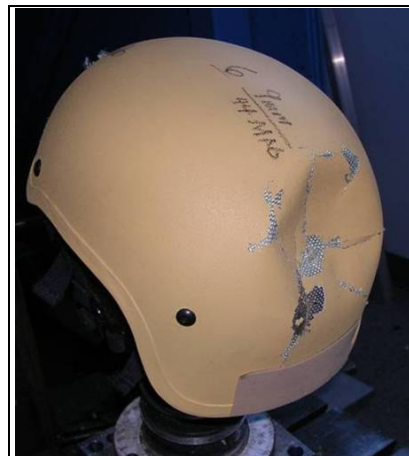
Figure 1: Shell deformation from a defeated handgun bullet.
