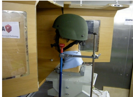
Figure 5. Test configuration with Large ACH helmet facing airflow (from left)
