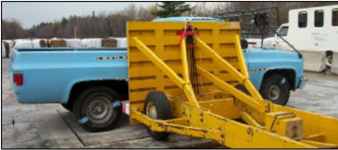
Figure 2. Alignment of the FMVSS 301 barrier for side collision.
