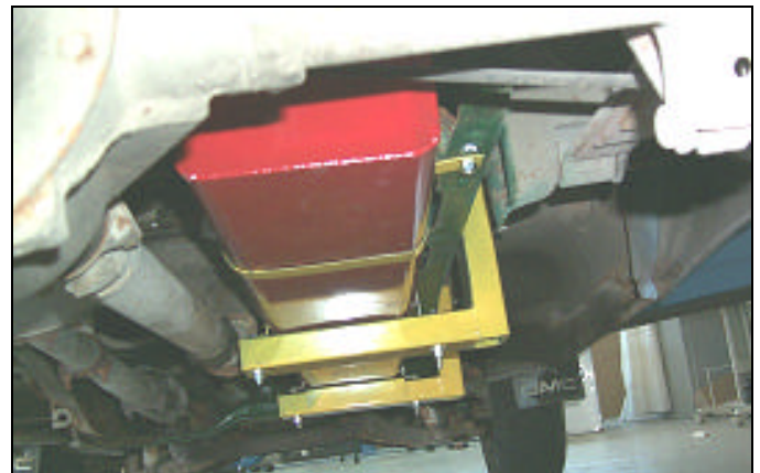
Figure 6. Typical center-mounted tank installation – rear view.
