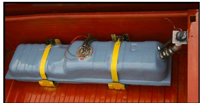
Figure 3. OEM bed tank installation with OEM brackets.
