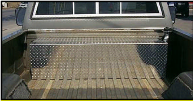
Figure 4. Typical in-bed installation of an OEM tank with shield
