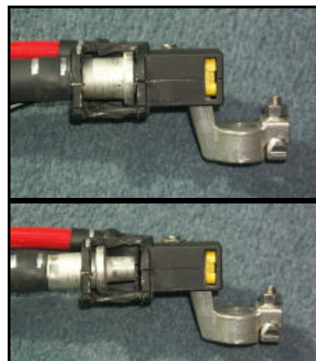
Figure 2: Cut-away view of a pyrotechnic battery disconnect.
