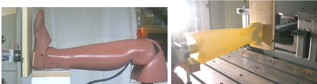
Fig. 8 – Funk-style Hybrid III (left) and CLL (right) test set-up
