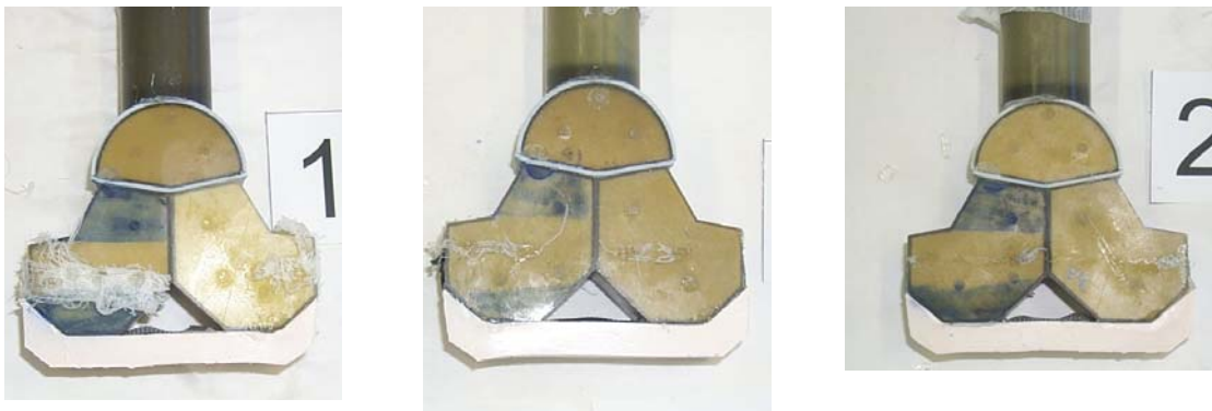
Fig. 7 – CLLs (with gelatin removed) after Owen-style testing
