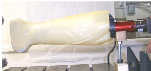
Fig. 11 – CLL set-up with the tibia load cell
