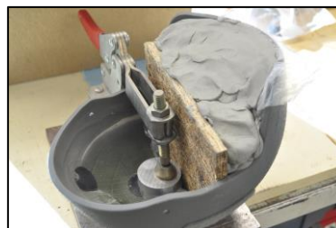
Figure 3. Helmet shell filled with clay witness material for qualification of BHBT.
