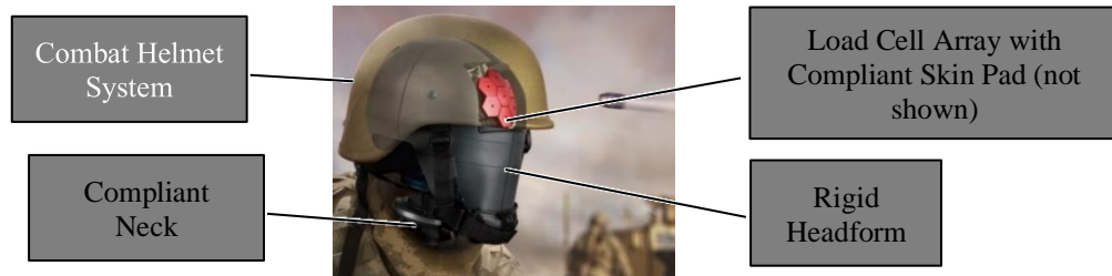
Figure 1: The Ballistic Load Sensing Headform for measuring BHBT.
