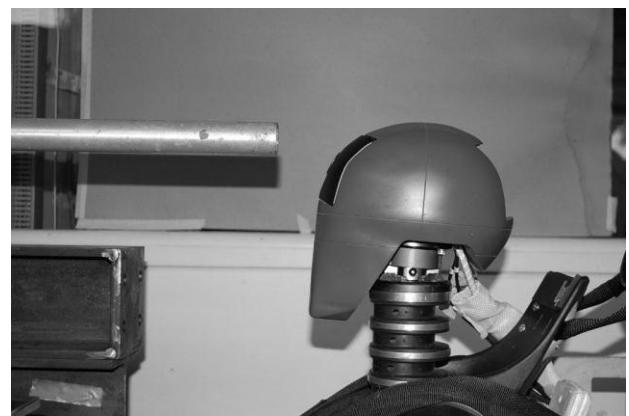
Figure 16: Ballistic cannon test setup. (Note the metal bar indicates the trajectory of the steel ball. Head protection was added afterwards.)
