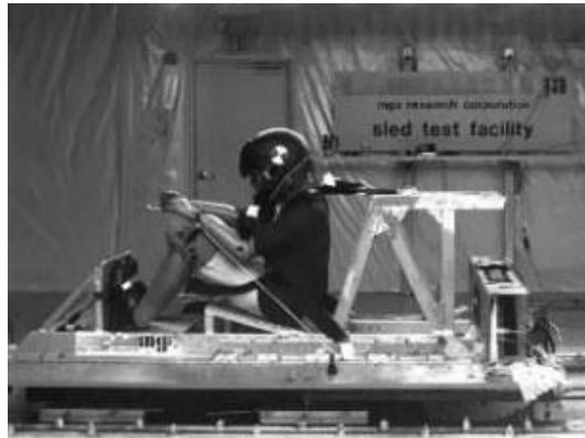
Figure 10: ATD with iHANS prototype at maximum forward excursion.
