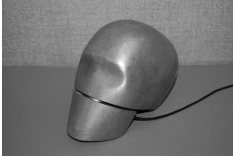
Figure 8: Hybrid III headform with force-sensing mandible section.
