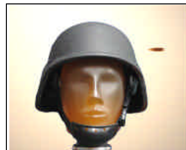
Figure 4: Ballistic helmet test with the instrumented headform.
