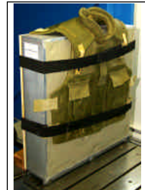
Figure 1: Body armour mounted onto a clay block for ballistics performance evaluation.
