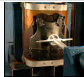
Figure 9: Torso impact membrane being used for blunt trauma assessment from impact.
