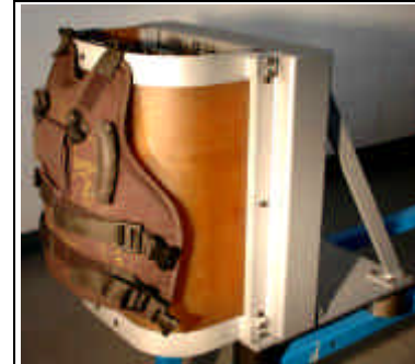
Figure 3: Body armour over the Thoracic Impact Membrane for blunt trauma assessment.
