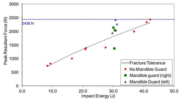
**Figure 6.** Peak resultant force for protected and unprotected impacts to the side of the jaw.
