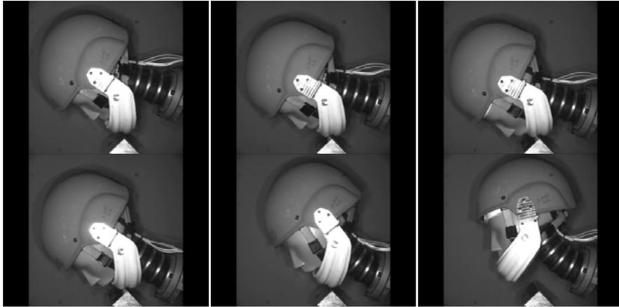
**Figure 8.** High-speed imaging of a 30 J blunt impact on the chin of the mandible guard.
