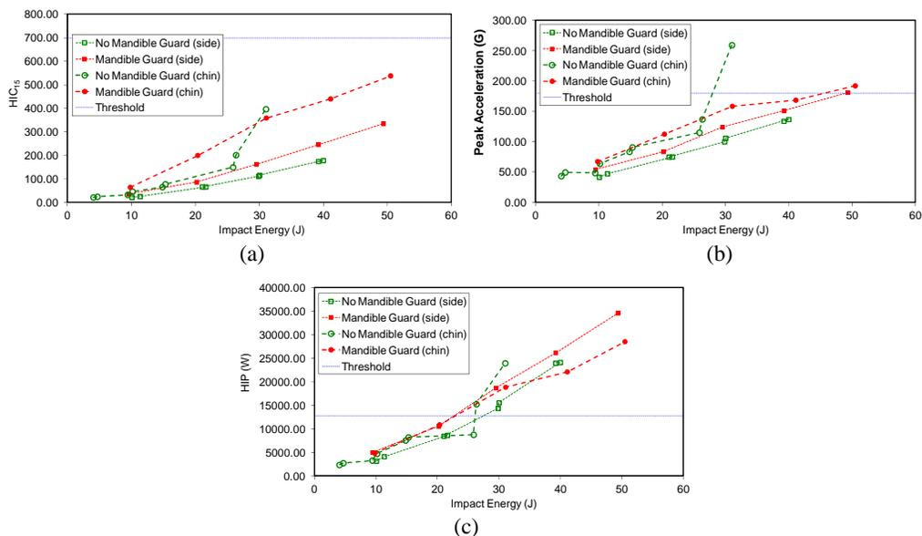
**Figure 12.** Head injury risk for protected and unprotected impacts to the chin and side of the headform: (a)  $HIC_{15}$ , (b) CG peak resultant linear acceleration, and (c) HIP.
