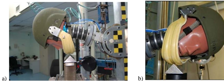
**Figure 3.** Setup for the blunt impact tests; a) frontal and b) oblique impact.
