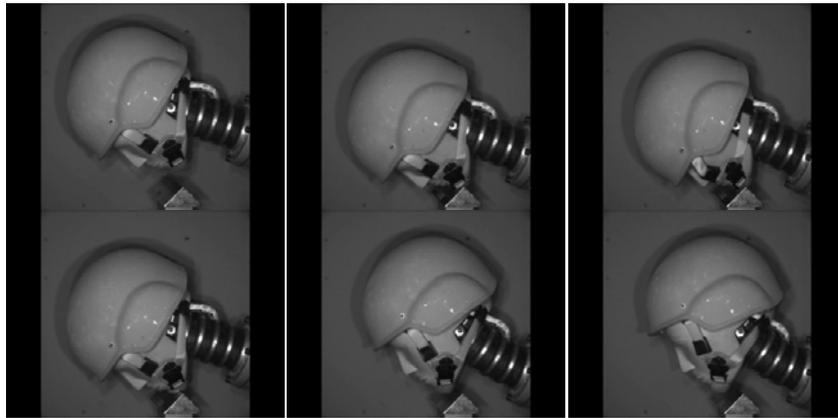
**Figure 9.** High-speed imaging of a 30 J blunt impact on the chin of the unprotected Hybrid III head.
