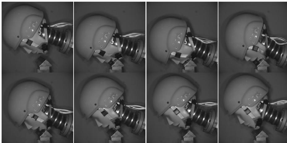
**Figure 7.** High-speed imaging of a 30 J blunt impact on the chin of the unprotected MLSH head.
