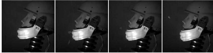
**Figure 13.** High-speed imaging of a ballistic impact over the chin.
