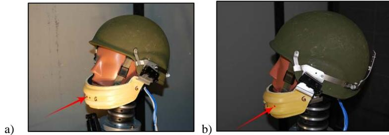
**Figure 2.** Behind armour blunt trauma test set-ups; a) strike to the chin; b) strike to the mandible body.
