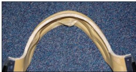
**Figure 14.** Typical residual backface deformation of the mandible guard (in this example, the strikes on the left and right sides were at lower velocity than over the chin).
