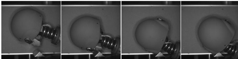
**Figure 10.** Example of torsional loading on the neck from a 30 J oblique impact to the mandible guard.
