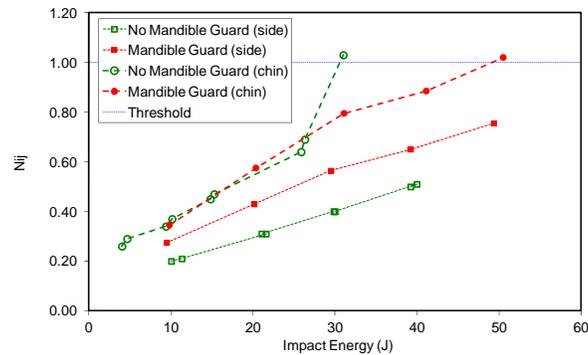
**Figure 11.** Neck injury risk as a function of impact load for protected and unprotected impacts to the chin and side of the headform.
