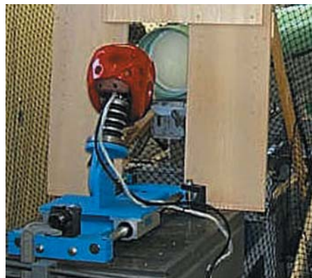
Figure 10 Test headform, air cannon and slider system (Kangaroo headgear installed).
