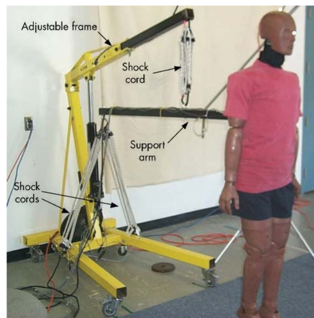
Figure 2 Hybrid III test manikin and support fixture.
